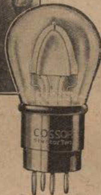
Below: A Stentor Two Valve used for this test.
